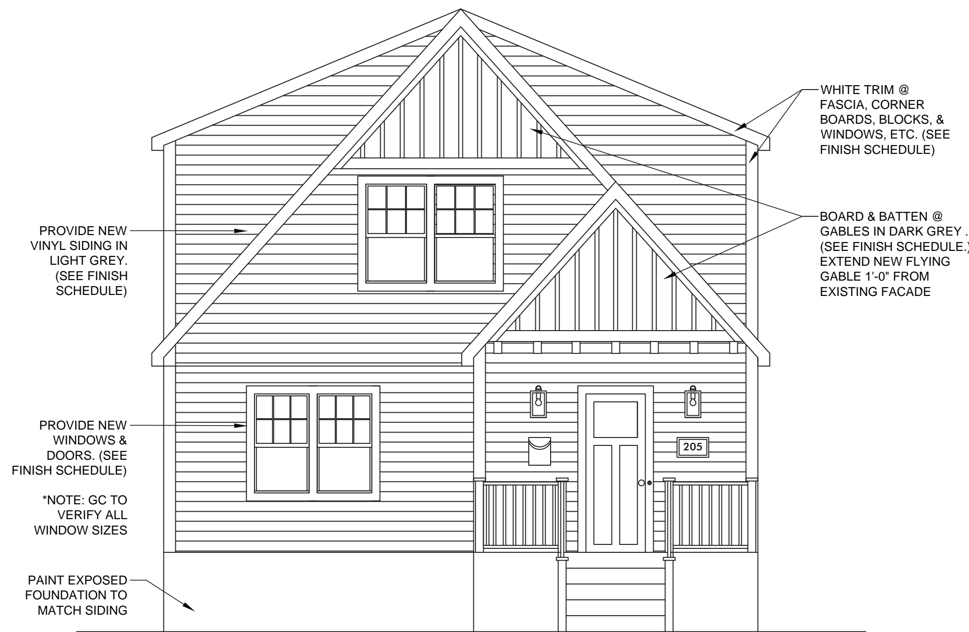
1 PROPOSED FRONT ELEVATION 1/4"=1'-0"
